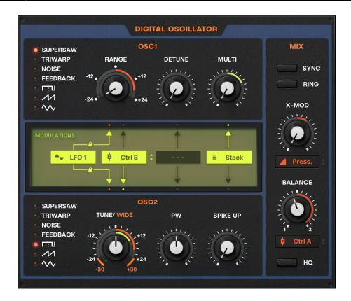
Digital OSC is the most drastically revamped section among OSCs. Basically it follows the "ring & box" modulation system, But since Digi OSC adopts "1 source - 2 targets" mod system, it looks a bit complicated.
